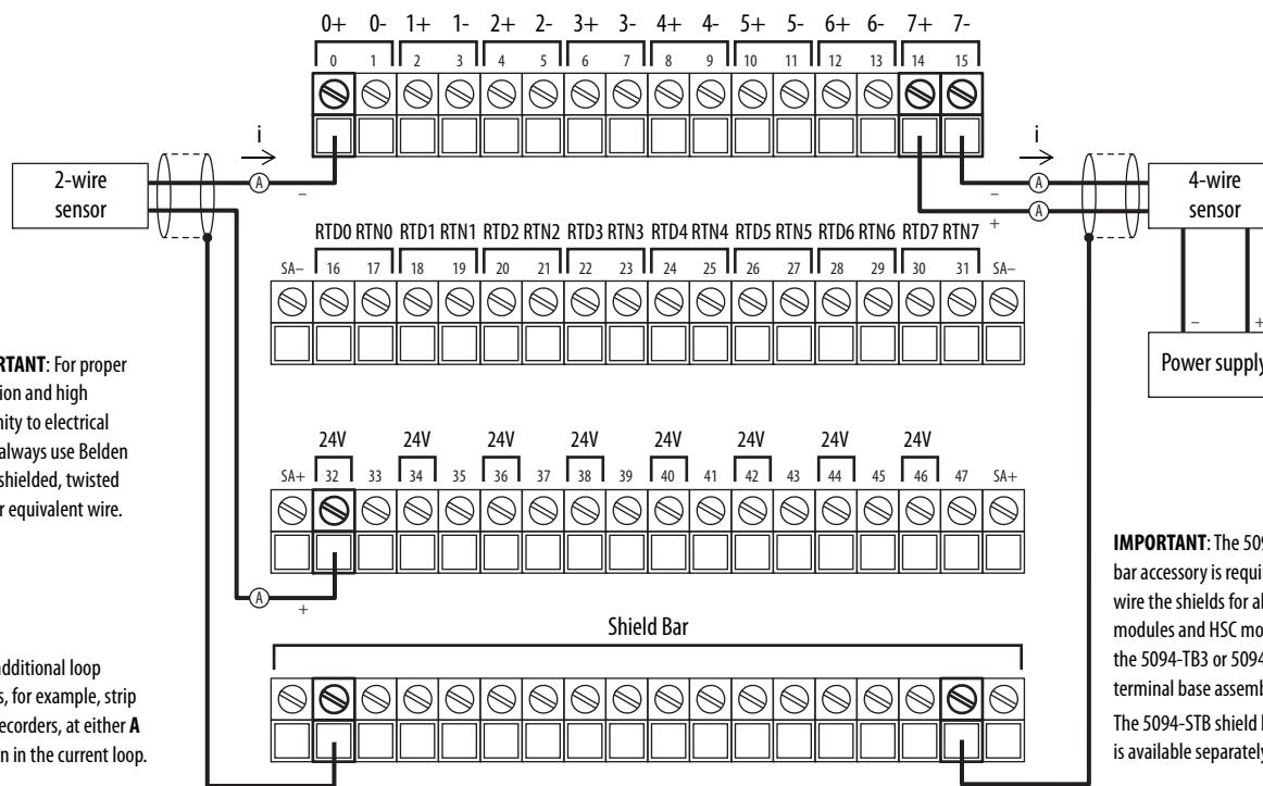
This figure shows a wiring diagram for the 5094-IY8 and 5094-IY8XT modules when used in voltage mode. You must connect a 24V DC power source to the left SA+/- terminals to provide field-side power.
