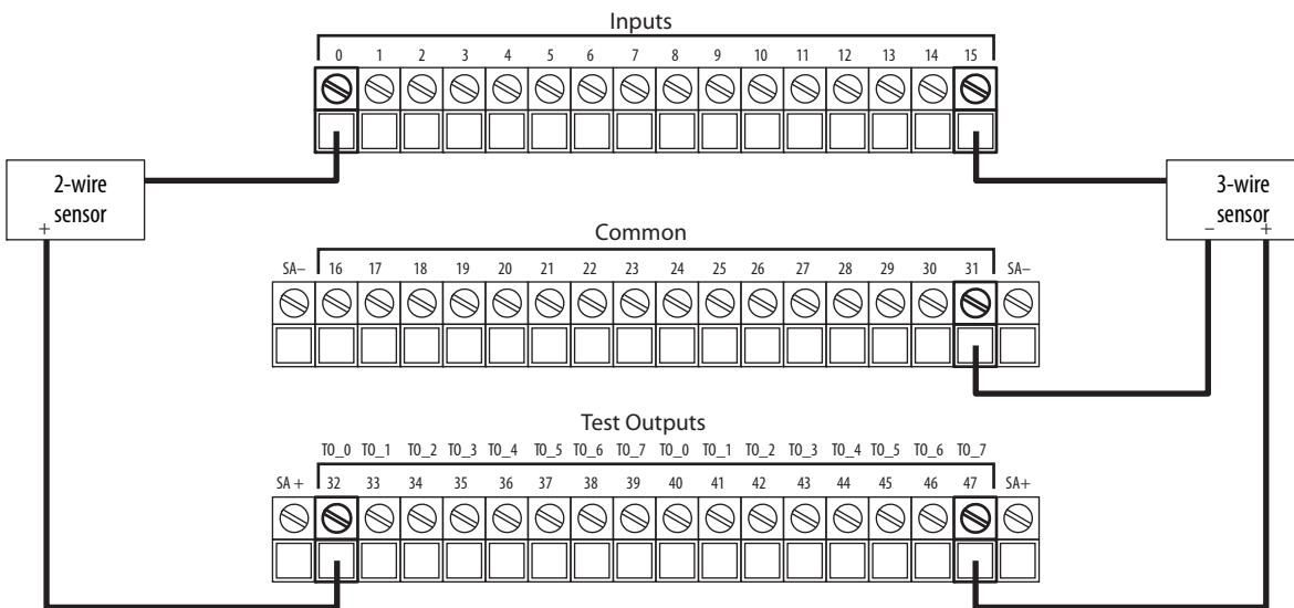
**IMPORTANT:** The 5094-IB16S module inputs use a shared common. The inputs have a return through internal module circuitry to the SA (-) terminal on the terminal base.
