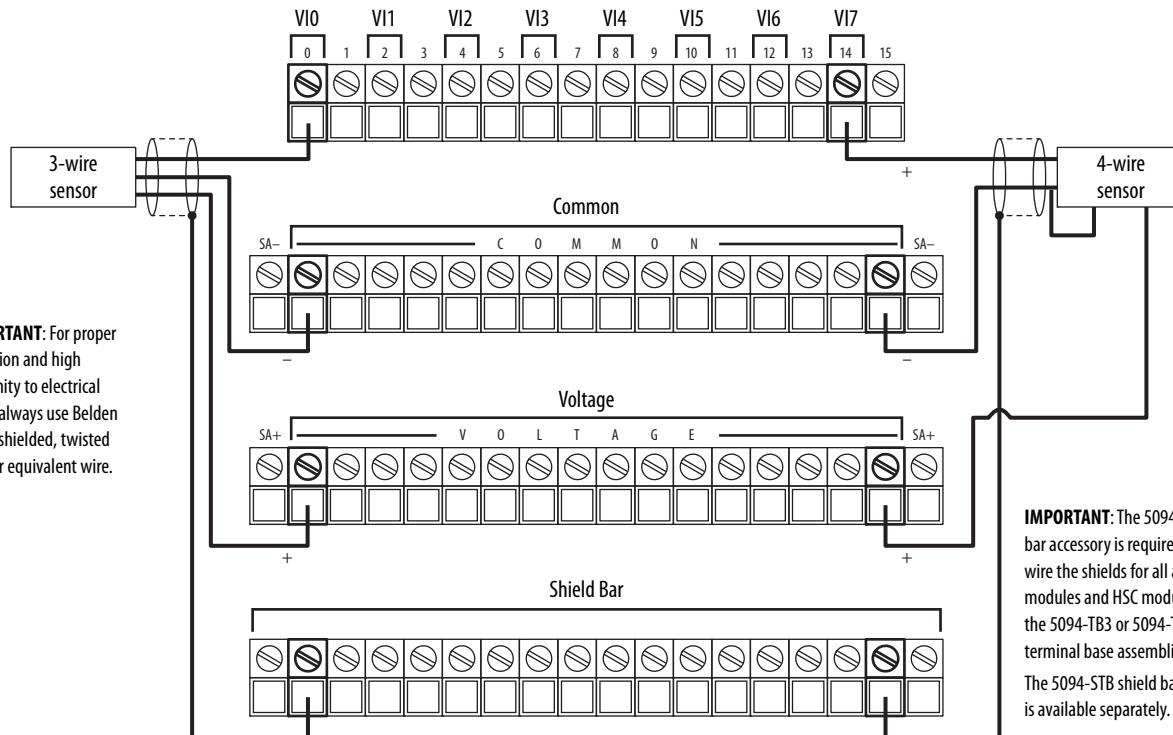
**IMPORTANT:** For proper operation and high immunity to electrical noise, always use Belden 8761 (shielded, twisted pair) or equivalent wire.
