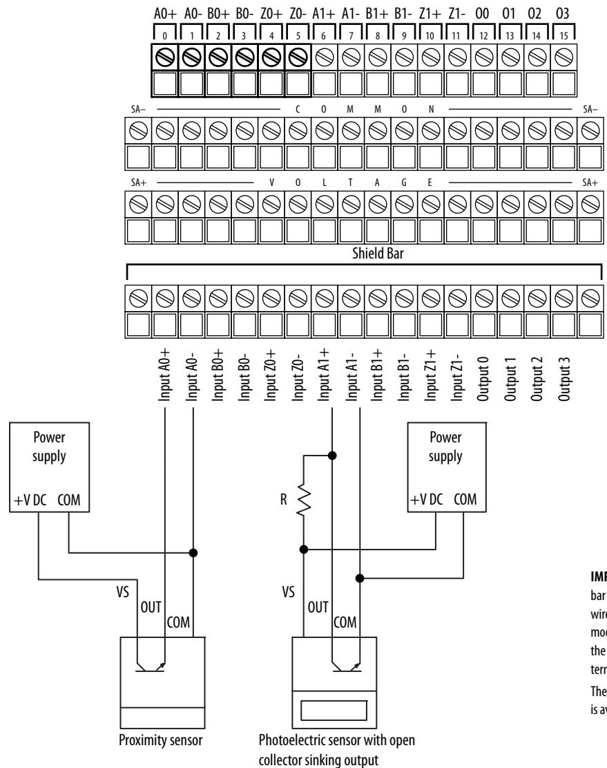
This figure shows a wiring diagram for the 5094-HSC and 5094-HSCXT modules connected to a discrete output device. You must connect a 24V DC power source to the left SA+/- terminals to provide field-side power.
