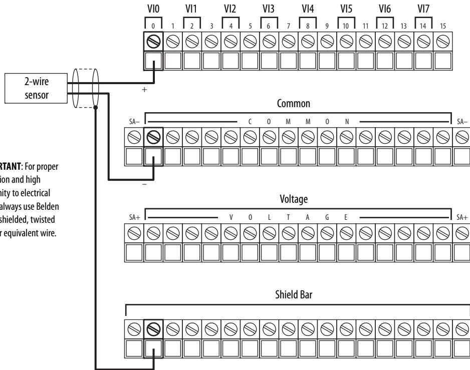
**IMPORTANT:** For proper operation and high immunity to electrical noise, always use Belden 8761 (shielded, twisted pair) or equivalent wire.
