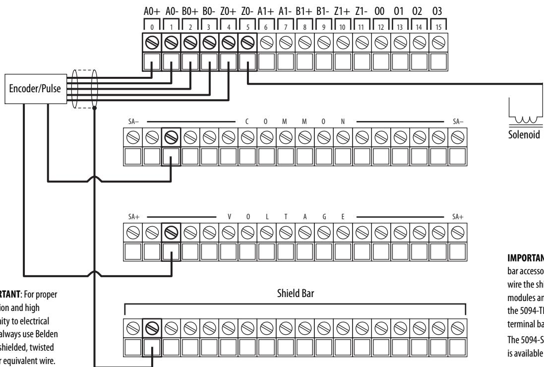
**IMPORTANT:** The 5094-STB shield bar accessory is required in order to wire the shields for all analog I/O modules and HSC modules using the 5094-TB3 or 5094-TB3T terminal base assemblies. The 5094-STB shield bar accessory is available separately.
