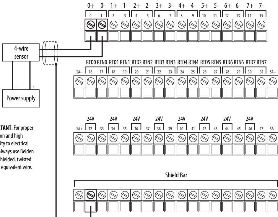
**IMPORTANT:** The 5094-STB shield bar accessory is required in order to wire the shields for all analog I/O modules and HSC modules using the 5094-TB3 or 5094-TB3T terminal base assemblies.
