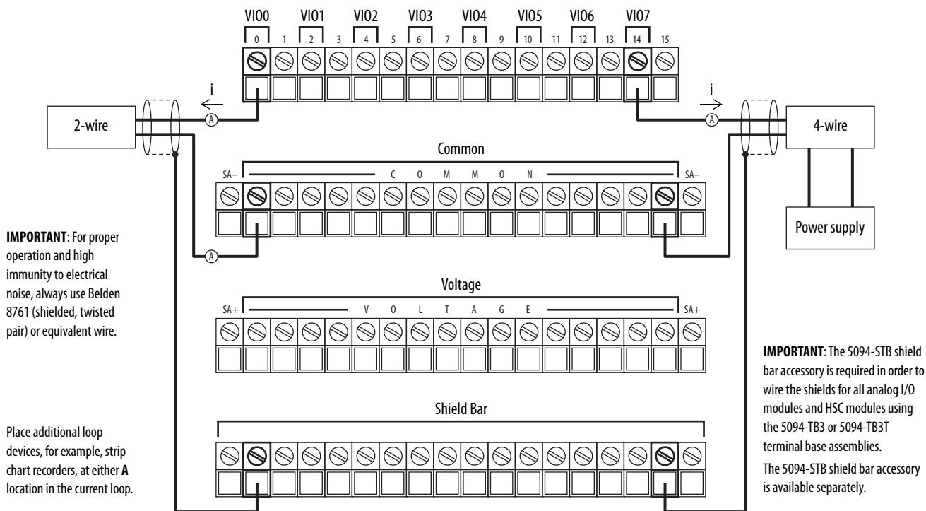
This figure shows a wiring diagram for the 5094-OF8 and 5094-OF8XT modules when used in voltage mode. You must connect a 24V DC power source to the left SA+/- terminals to provide field-side power.
