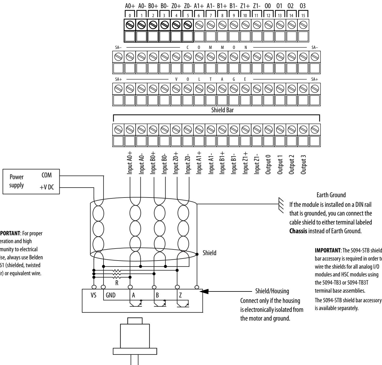
This figure shows a wiring diagram for the 5094-HSC and 5094-HSCXT modules connected to discrete input devices. You must connect a 24V DC power source to the left SA+/- terminals to provide field-side power.
