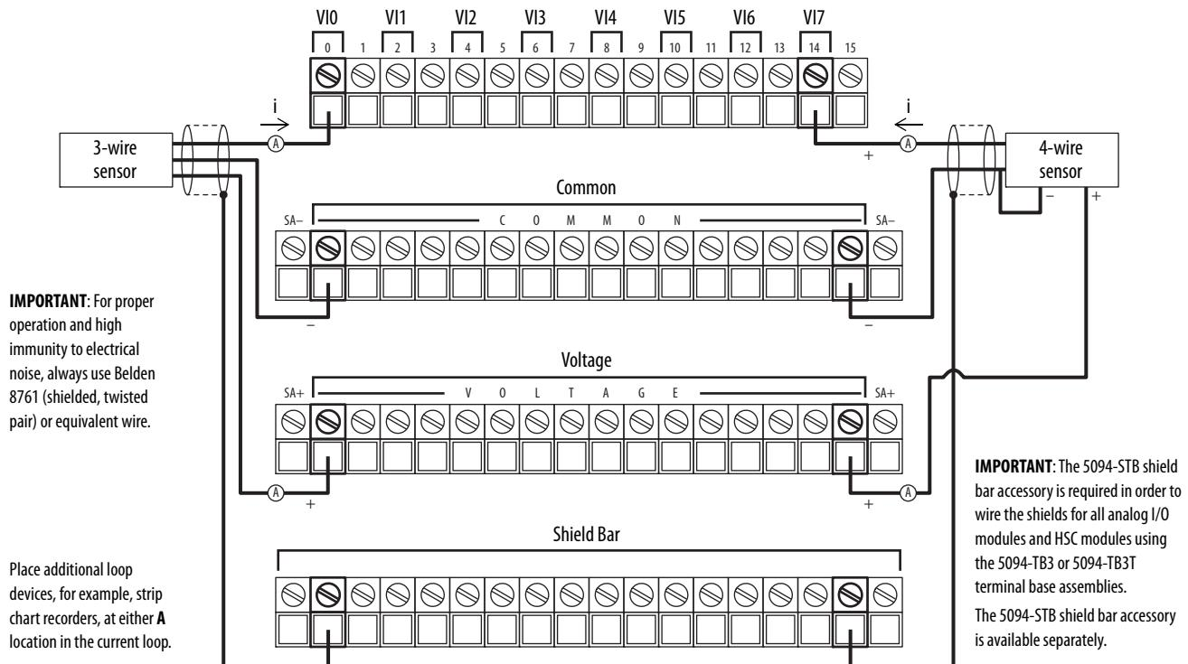
This figure shows a wiring diagram for the 5094-IF8 and 5094-IF8XT modules when used in voltage mode. You must connect a 24V DC power source to the left SA+/- terminals to provide field-side power.
