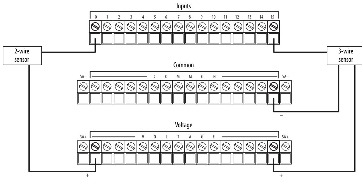
**IMPORTANT:** The 5094-IB16 and 5094-IB16XT module inputs use a shared common. The inputs have a return through internal module circuitry to the SA (-) terminal on the terminal base.
