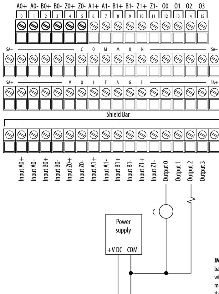
**IMPORTANT:** For proper operation and high immunity to electrical noise, always use Belden 8761 (shielded, twisted pair) or equivalent wire.
